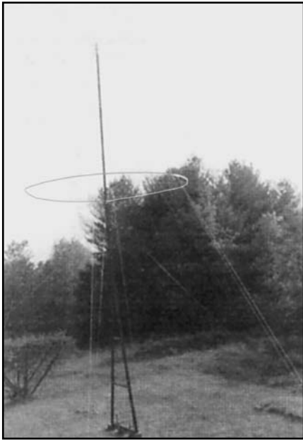
Fig 50—Photo of W8NWF's original A-frame mounted HF disc.
